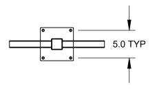
6"X6"X0.25" SQUARE FLANGE MOUNTING PLATE WITH 4  $\,$   $\,$  3/8" MOUNTING HOLES
