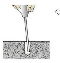
Tool to remove debris after drilling holes. Installer provides.
