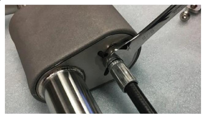
Wrap threads of new hose with PTFE tape. Wrap all threads, 2 to 3 full turns.
