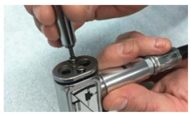
2 Note orientation of seals in the pump head.
