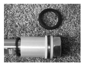
19. Remove rod wiper seal using a pliers. Be careful not to damage plastic. Replace wiper seal (Kit Item 'l'). Be careful not to damage the seal.
