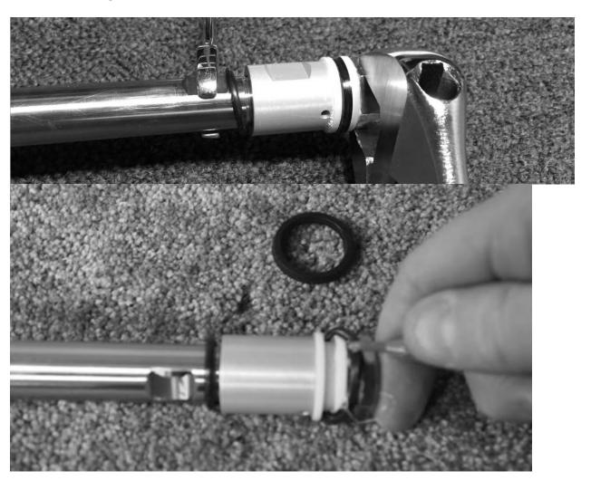
16. Remove piston using a 16mm wrench and an adjustable wrench.
