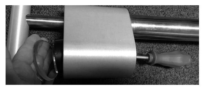
5. Using a 13mm socket, remove the two gauge housing retaining bolts.
