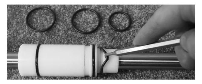
21. Remove and replace the gauge housing O-rings. (Kit item 'A')
