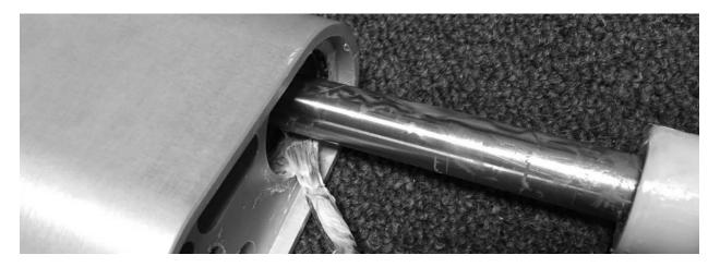
24. Grease top of Pump Cylinder (Bottom Bumper should still be in the bottom of the Pump Tube).
