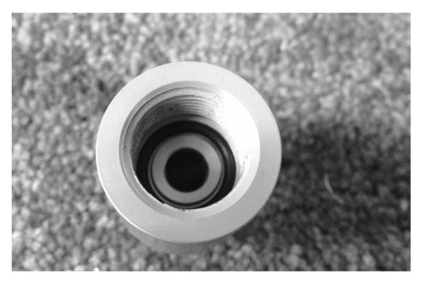
18. Replace O-ring on piston (Kit Item 'L'), piston seal (Kit Item 'J'), and wear ring (Kit Item 'G'). Note the piston seal sits, with the open end towards the bottom of the pump. Place bushing on rod. Do not forget to replace upper bumper (Kit Item 'N') Tighten Piston housing and Piston nut.
