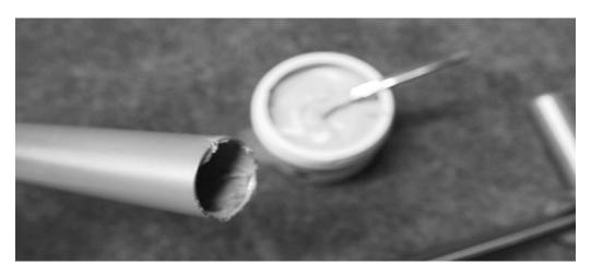
25. Slide Piston and Pump Rod into Pump Tube. Start with piston at an angle, taking care not to damage the Rod Wiper Seal or force it to fold while entering the tube. It may help to gently guide the Rod Wiper Seal into the pump tube by using your finger nail or a soft plastic hook tool.
