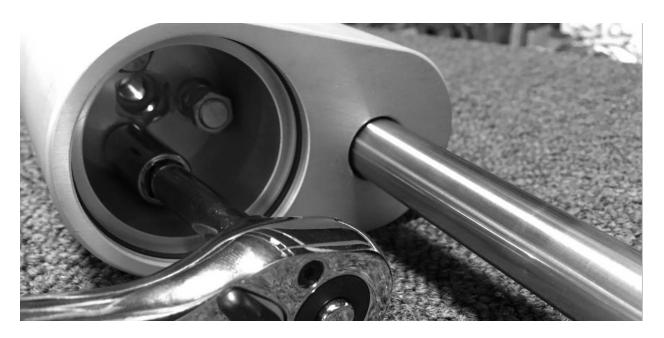
6. You can now remove the contents of the pump. First pull up on the gauge housing. Due to the O-rings on the housing, this may be tight and require some light taps with a plastic/rubber hammer. When that is loose, you can now stand on the pump housing flange and pull the handle out. Due to the O-rings on the bushing, this may also be tight.
