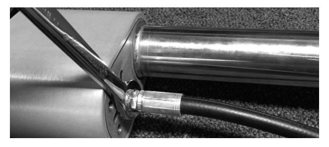
4. Insert a hex key or screwdriver into the bottom of the gauge housing to remove the gauge cover and pressure gauge. You may need to lightly tap with a hammer.
