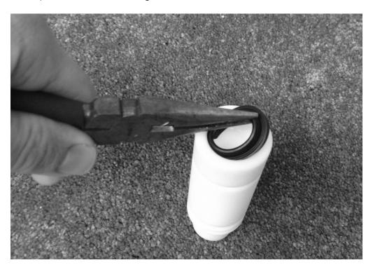
20. Remove o-rings that are to be replaced on the bushing. Replace with new O-rings (Kit Item 'P' and 'K'). Take care not to damage the o-rings on any material edges they may have to go over.
