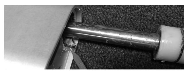
22. Re-grease O-rings on Bushing. Place a thin layer of grease below the bushing on the Pump Rod.
