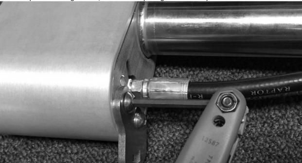
3. Remove the air hose from the bottom of the gauge housing using a 9/16" (14mm) wrench.
