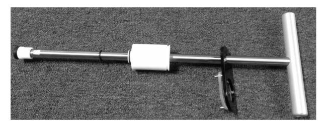
9. Replace bushing O-ring and upper bumper O-ring with the replacements in the kit.
