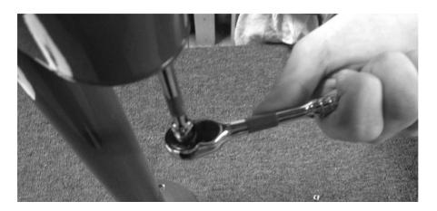
4. When all three nuts have been removed, pull the top cap off the pump. You can now lift the pump rod, bushing, and cylinder out of the pump. There is a tubing attached to the bottom of the pump. Be careful not to kink this line while removing the internal components.
