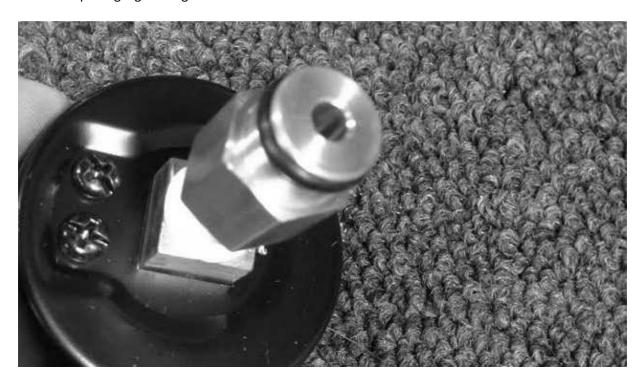
8. You can now remove the piston and rod from the cylinder.
