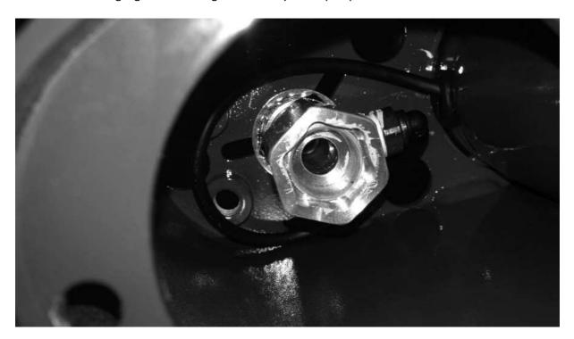
21. Connect the tubing to the footvalve.
