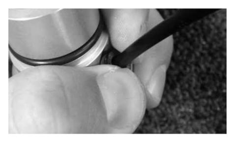
22. Begin installing the pump's internal components into the housing as shown. **NOTE: Slowly install assembly to avoid kinking the tubing.**
