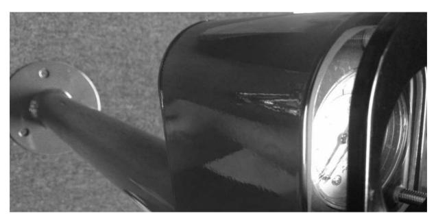
26. Install and tighten the nuts to the top cap. To make this easy, load a socket as shown so that the threads are easily started.
