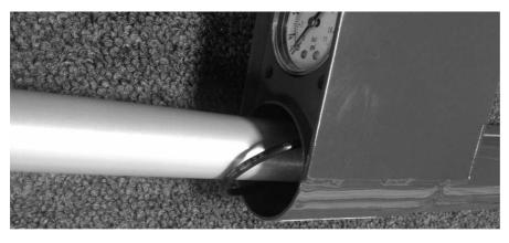
23. You will lower the assembly down. To keep the components from separating while lowering it into the pump housing, you will grab the piston rod, bushing, and cylinder while lowering as shown.
