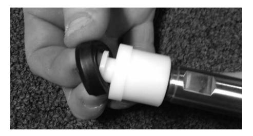
11. Lubricate new piston seal with provided grease.
