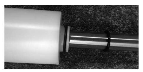
10. Replace the piston seal by hand. The new seal can also be installed by hand.
