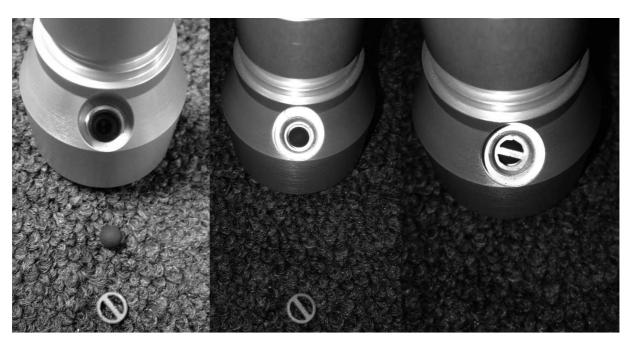
17. Apply thread sealing tape to fitting and reinstall with 1/8" hex key.
