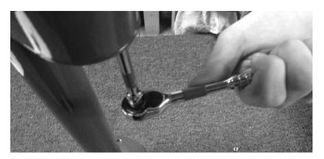
28. If you need to replace the hose, use a large adjustable wrench and a 9/16" or 14mm wrench to remove the hose. **NOTE: Do not attempt to remove hose without an adjustable wrench to react the torque or the gauge will spin.**
