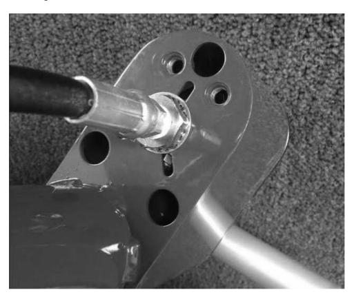
3. Using a  $\frac{1}{4}$ " drive ratchet with a 6" long extension and a 10mm socket, remove the three top cap nuts.
