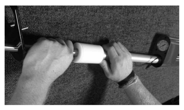
5. In order to disconnect the air line from the foot valve at the bottom of the pump, you must depress the tabs of the fitting and then pull on the hose.
